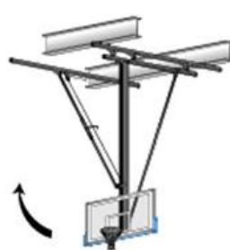
Side Fold (over retractable seats or to stop overhead interference of main court from cross court structure)
